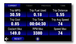
The TODAY's trip can manually be changed to start a new day if the ScanGauge didn't recognize a new day started by pressing NEW DAY at the bottom. This will force the TODAY trip into the PREVIOUS day.
