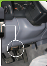
Typical OBDII Connector location
